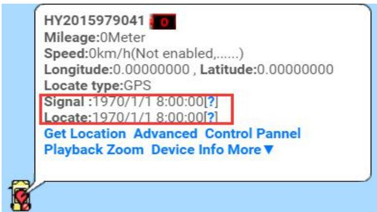
**NOTE:** If you insert the correct SIM card and open GPRS. device in outdoor,login the app,as above picture,the address and time are incorrect,device did not upload location to APP, Please set the APN commands
